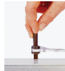
No.3 Turn broken screw out steadily without tilting
