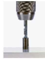
No.1 Drill into broken thread with drilling jig
